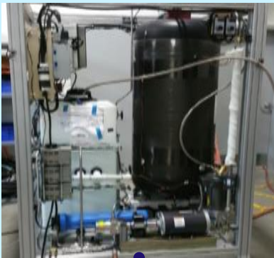
Ground Level Integrated Diverse Energy Storage (GLIDES) prototype since 2019. Efficiency from 70% to 82%
