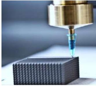
Production of 3D structured catalyst through micro-extrusion of a ceramic/metallic paste to built a porous material (VITO)
