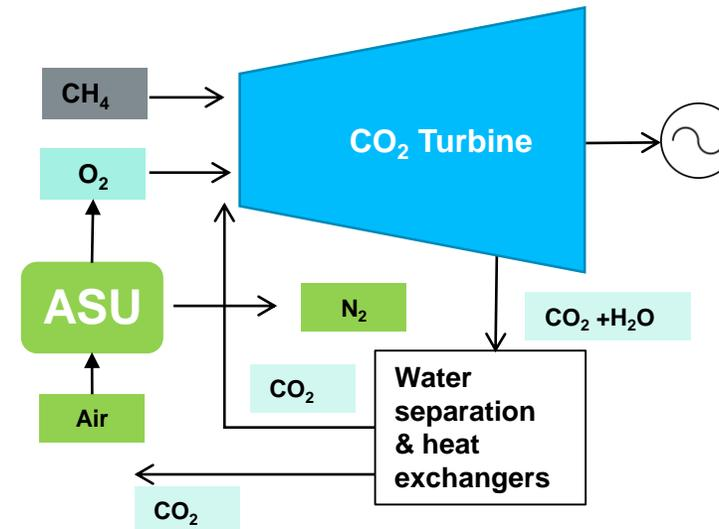
With NG, efficiency rate expected is 59%, similar to CCGT plus exhaust flue gas with 90% CO<sub>2</sub> concentration.
