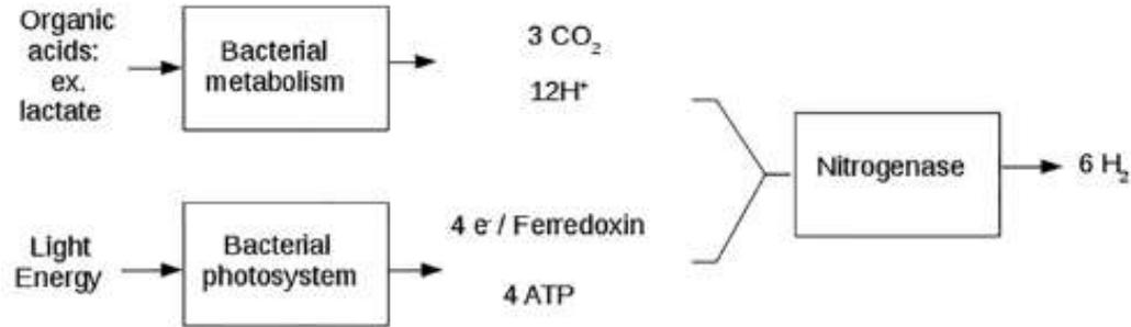
Main pathways of hydrogen production by photofermentation of organic acids by using photosynthetic bacteria
