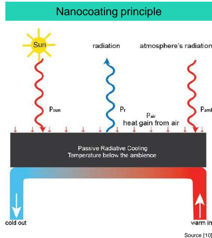
**Thermal balance of cooling**
