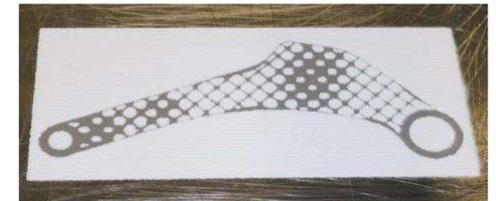
Aerosint's concept technology for selective deposition of powder on 3D printing machine build platform, showing co-pattern of titanium (grey powder) and polymer PA12 (white powder)
